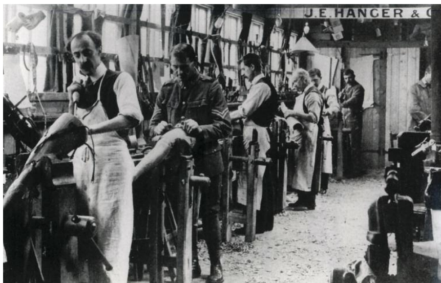
Civil war amputee James E. Hanger, left, developed a prosthetic leg hinged at knee and ankle. Workers produced the Hanger Limb at his workshop, right. Above: A diagram accompanied Hanger's first U.S. patent, issued in 1871.
